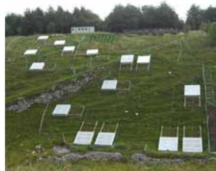
Automatic retractable rain-shelters in position over fifteen drought treatment plots in July
